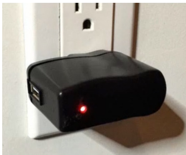
Figure 7.7 – A keylogger hidden inside a USB charger
