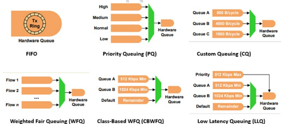
Figure 15-11. Graphical representation of QoS queuing types
