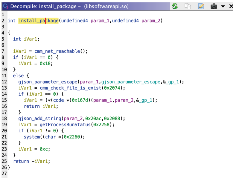
Figure 5.22 – The install_package function
