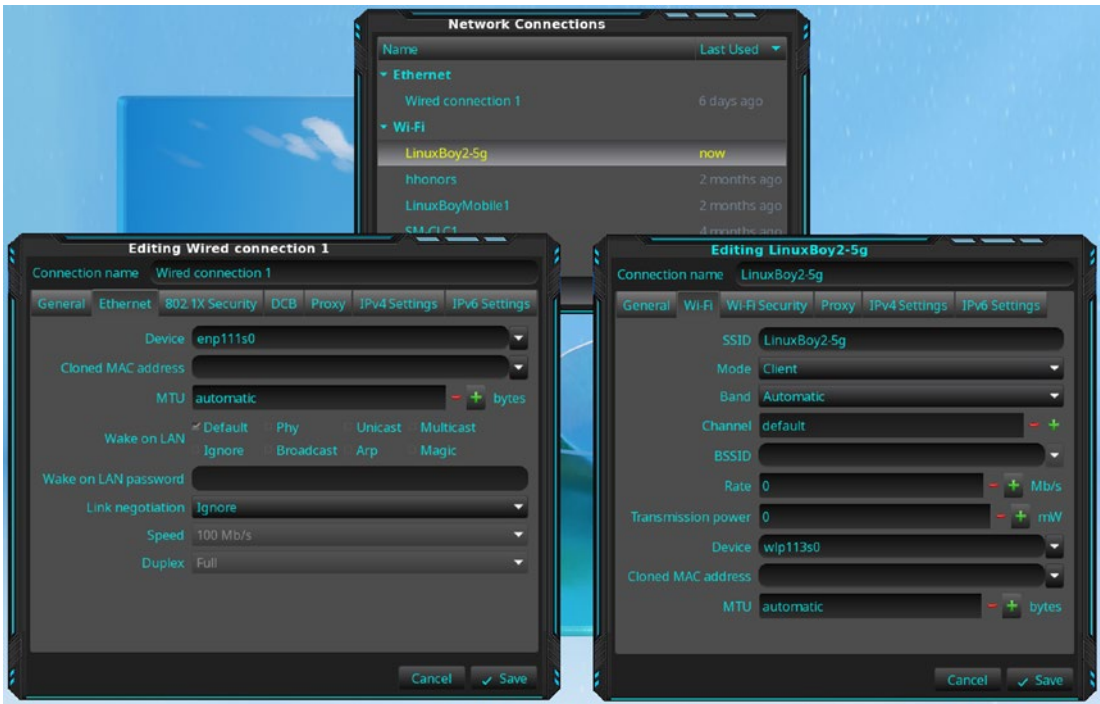
Figure 33-5. Both wired and wireless connections can be viewed and edited using the GUI connection editor
