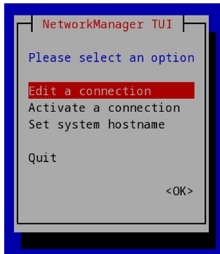
Figure 33-2. Using nmtui, select Edit a connection to create a new keyfile
