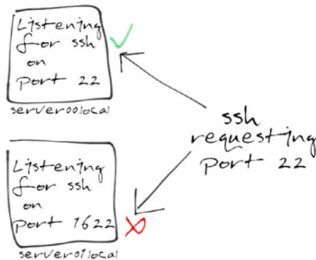
Figure 41-1. An SSH – or any other – connection can only be made if the server is listening on the correct port
